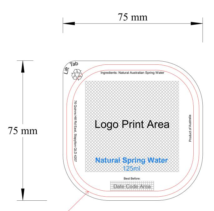
The 2 x RED lines indicate the weld ring where the cup lid is welded to the cup.
